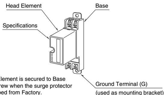
Head Element is secured to Base with screw when the surge protector is shipped from Factory.
