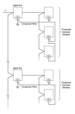
1. Fieldbus devices complying with IEC 61158-2 operate by a supply voltage between 9V and 32V DC. Take the MDP-PA's internal series resistance into consideration when determining the
