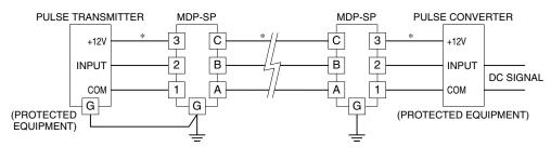
\* When there is no need of power supply, the cable is also unnecessary.
