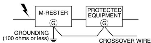
A crossover wire between M-RESTER ground and the ground or metallic housing of the equipment is required for protection. If the protected equipment has no ground terminal, ground the M-RESTER only. When the M-RESTER is mounted with DIN Rail Mounting Adapter, connect the grounding wire to the mounting screw of the M-RESTER.
