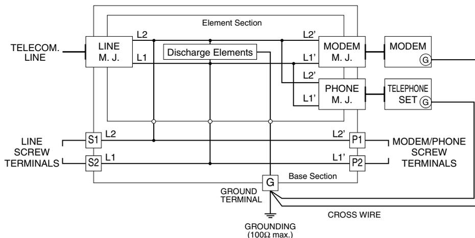
Be sure to cross-wire between G terminals of modem / telephone set and the G terminal of the MDP-TL.
