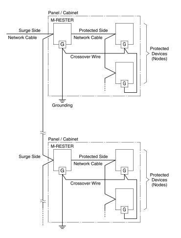
• The M-RESTER is applicable to networks which consist only of FTT-10A.
