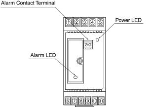
The MDW5ALW consists of a head element and base. The head element incorporates surge suppression circuit, life monitoring circuit and a battery for memorizing the life. The base incorporates power circuit and a relay for alarm output. When the surge suppression circuit is damaged or the battery is weakened, replace the head element to recover the surge protector's performance. Replacing the head element does not disturb the communication.
