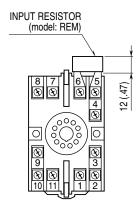
Input shunt resistor attached for current input.
