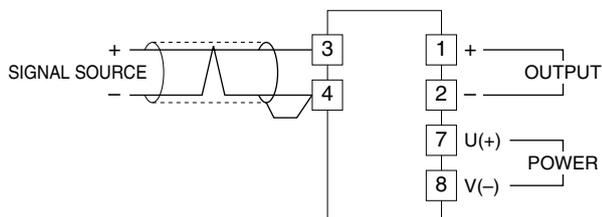
The MLG is designed to amplify very low level signals by high gain. In order to prevent the output becomes unstable due to input noises, use shielded twisted-pair cables or take other precautions for input wiring.
