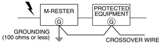
A crossover wire between M-RESTER ground and ground or metallic housing of equipment is required for protection. If the protected equipment has no ground terminal, ground the M-RESTER only.
