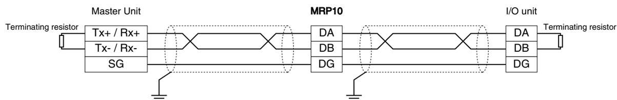
Terminating resistors can be turned ON/OFF on the PC configurator software (model: STCFG) or programming unit (model: PU-2x).
