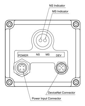
Figure 3. Component identification, Communication Box
