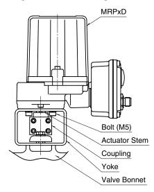
Figure 7. MRP×D mounted onto a valve (example)
