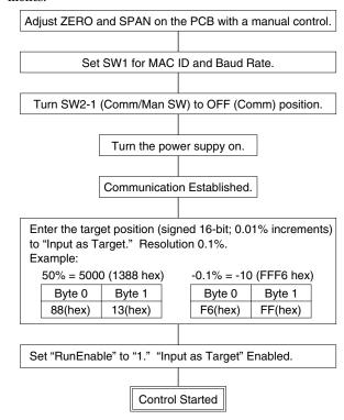
Once the communication is established, the actuator can be operated only by setting "RunEnable" and providing "Input as Target."
