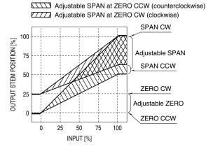
Figure 5. I/O characteristics (adjustable range)
