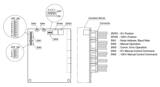
Figure 4. Component identification, Control PCB
