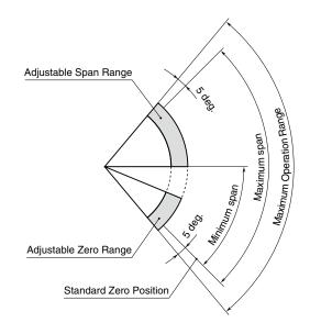
Figure 6. Definition of the minimum and maximum spans
