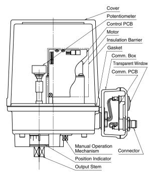
Figure 2. Component identification, MRP6D
