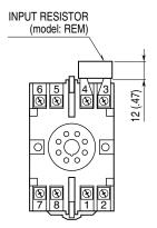
Input shunt resistor attached for current input.
