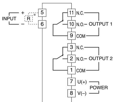
\*Input shunt resistor attached for current input.
