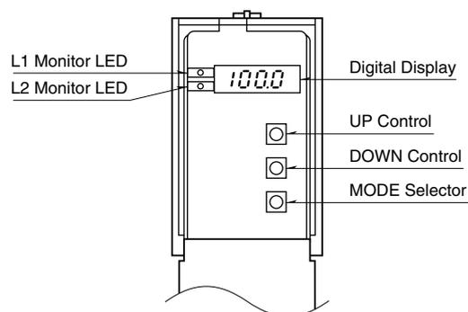
The MSEF has three function modes for checking and programming parameters:
