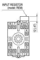
Input shunt resistor attached for current input.
