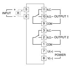
\*Input shunt resistor attached for current input.
