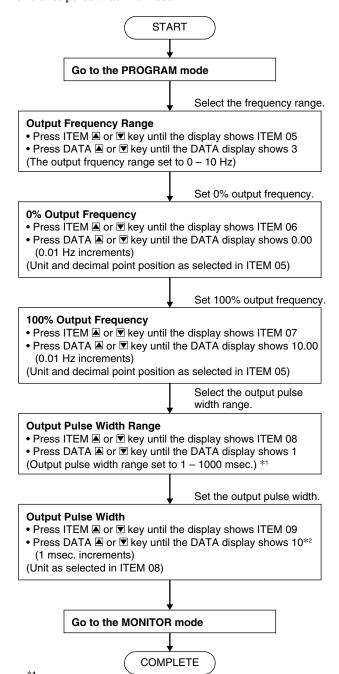
$^{*2}$  50 – 1000 msec. for AC/DC switch output. If the selected pulse width is greater than the cycle at 115% output, the MXAP does not function adequately. (ITEM 09 data blinks with an abnormal setting.)
