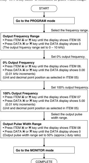
[Example 2] Output frequency range 0 to 10 Hz One-shot pulse width 10 msec.
