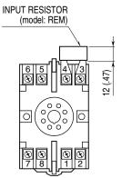
Input shunt resistor attached for current input.
