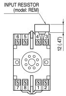
Input shunt resistor attached for current input.
