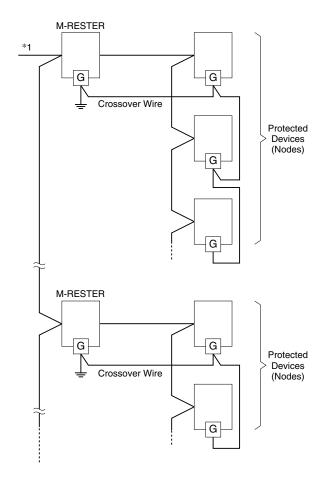
\*1. Fieldbus devices complying with IEC 61158-2 operate by a supply voltage between 9V and 32V DC.
