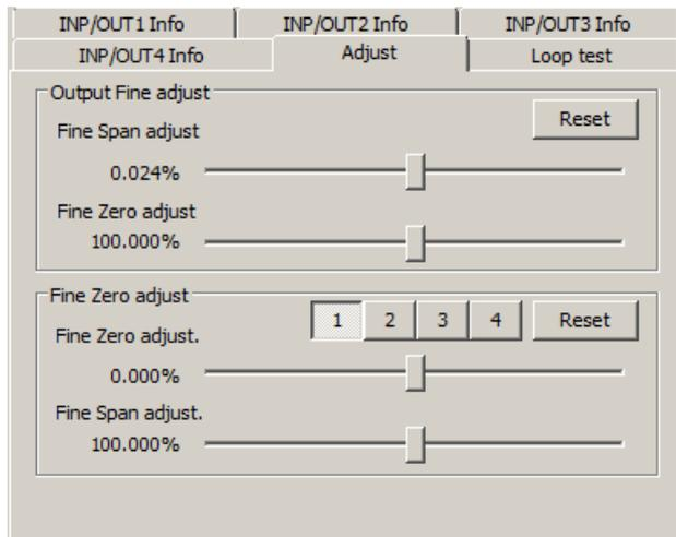
Perform 'Input Fine adjustment' while monitoring the input value indicated on the display of the device or the input value indicated on the upper part in the [Device Configuration] frame of the M1E1CFG.
