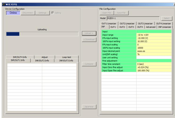
When the download is complete, the setting parameters edited in the [File Configuration] frame are written into the device.
