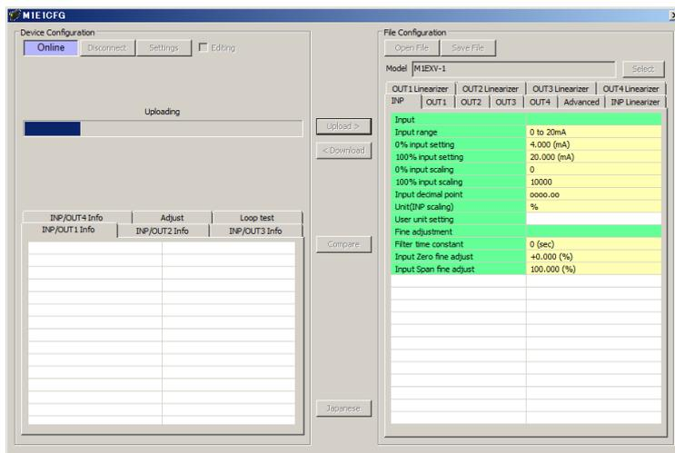
When the upload is complete, the parameters are shown within the [File Configuration] frame and become editable.
