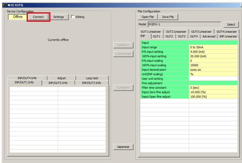
The model of the device is automatically recognized and the device data is uploaded and shown in the [Device Configuration] frame.
