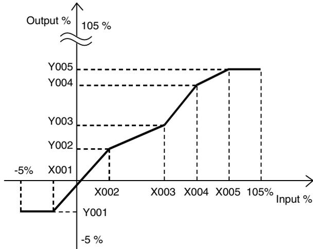
When the input to be converted does not match any X value in the table, two X values which are closest to the input in positive and negative directions are selected and linearly interpolated, thereby obtaining a Y value to be outputted.
