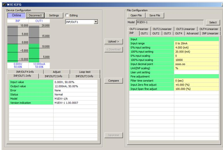
The bargraph shows real time I/O status of the device, and the I/O to display on the bargraph can be selected from the pull-down menu.
