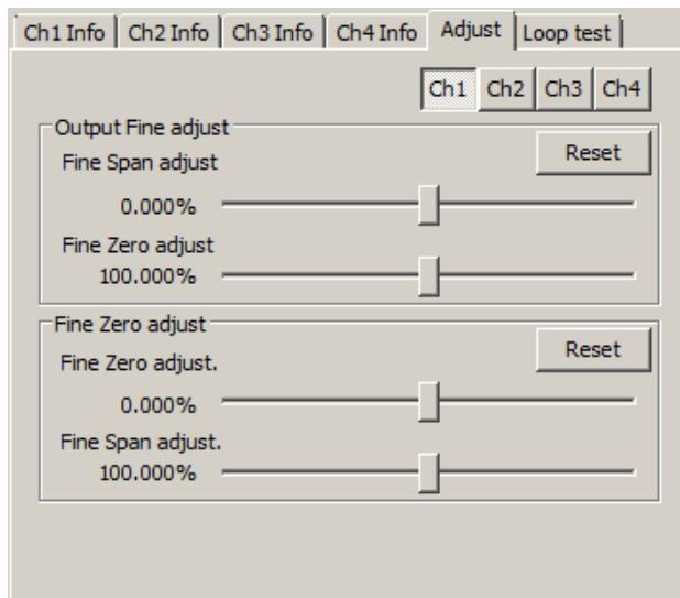
Perform 'Input Fine adjustment' while monitoring the input value indicated on the display of the device or the input value indicated on the upper part in the [Device Configuration] frame of the M1E4CFG.
