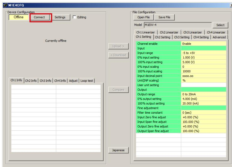
The model of the device is automatically recognized and the device data is uploaded and shown in the [Device Configuration] frame.
