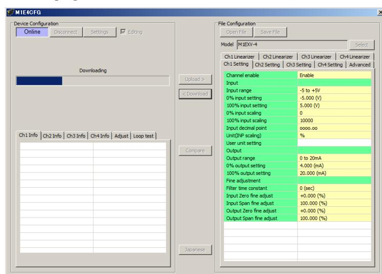
When the download is complete, the setting parameters edited in the [File Configuration] frame are written into the device.
