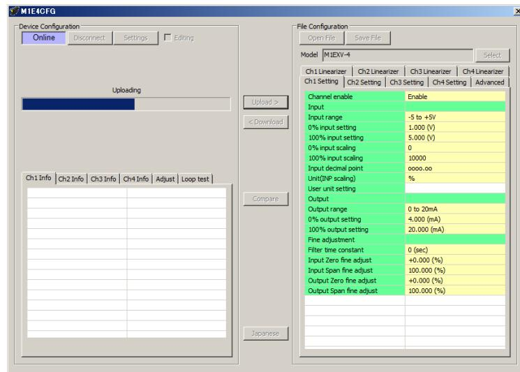
When the upload is complete, the parameters are shown within the [File Configuration] frame and become editable.
