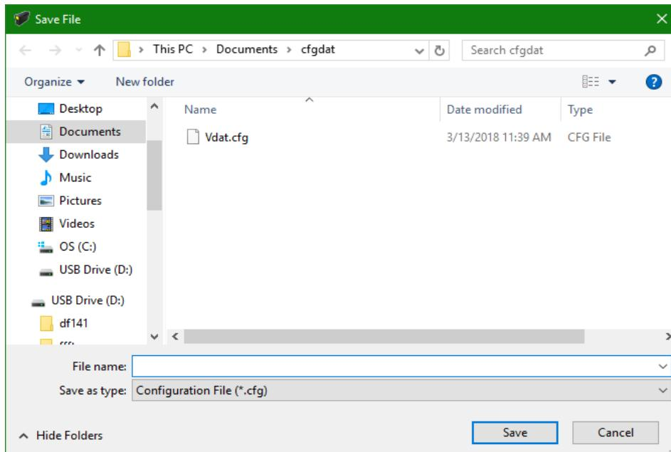
Enter a desired file name to File Name field and click [Save] to store the parameters in the [File Configuration] frame.
