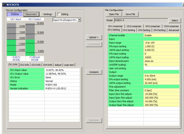
The bargraph shows real time I/O status of the device, and the I/O channel to display on the bargraph can be selected from the pull-down menu.
