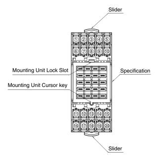
Note: The side of mounting unit lock slot have No. 1 – 10 terminal connections.
