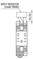
Input shunt resistor attached for current input.
