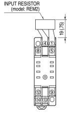
Input shunt resistor attached for current input.
