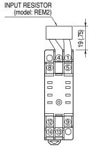
Input shunt resistor attached for current input.
