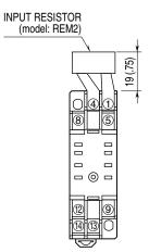
Input shunt resistor attached for current input.
