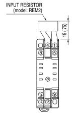
Input shunt resistor attached for current input.
