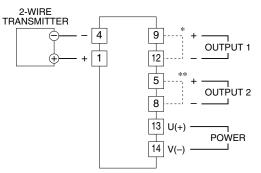
\* Short across these terminals for large voltage allowance at Output 2. Be sure to match specifications of smart transmitter. Do not connect a capacitive load to Output 1.
