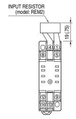
Input shunt resistor attached for current input.
