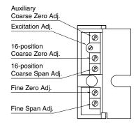
1) Excitation Adj.: The excitation voltage is calibrated at the factory, therefore will not usually require adjustment, except when used in combination with a strain gauge of sensitivity other than described on the specifications.
