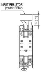
Input shunt resistor attached for current input.
