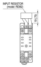
Input shunt resistor attached for current input.
