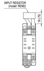
Input shunt resistor attached for current input.
