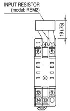
Input shunt resistor attached for current input.
