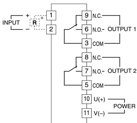
\*Input shunt resistor attached for current input.
