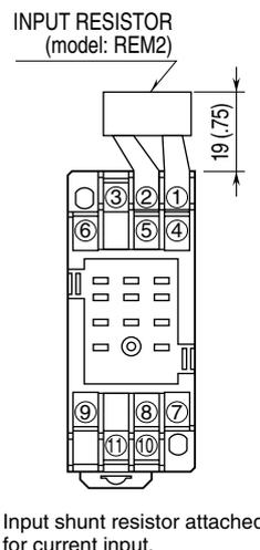
Input shunt resistor attached for current input.
