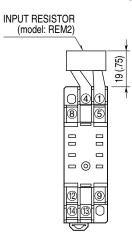
Input shunt resistor attached for current input.
