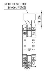
Input shunt resistor attached for current input.
