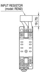
Input shunt resistor attached for current input.
