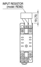
Input shunt resistor attached for current input.
