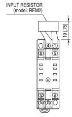
Input shunt resistor attached for current input.
