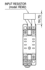
Input shunt resistor attached for current input.
