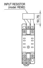
Input shunt resistor attached for current input.
