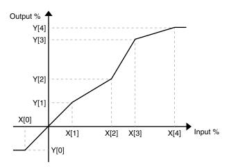
If a value equal to the input % value is not set in X[n], extract the closest value in each of the positive and negative directions from the set X[n], and then linearly complete the two points as shown in the formula below to obtain the output % value.
