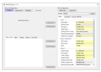
Connecting the compatible device to the PC via the configurator connection cable, the device model will be automatically recognized and the device information will be displayed as shown below.
