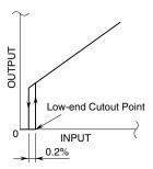
When the output low limit is set to a value higher than 0%, the input below the low-end cutout point is forced to the value, not 0%.
