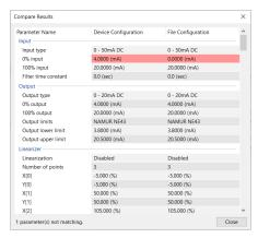
The compared parameters are displayed in the order of parameter name, device set value, and file set value for each line.
