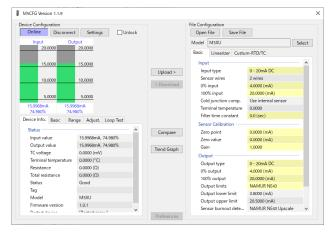
The I/O levels of the device are displayed in a bar graph. Various operations can be performed from the each tab, "device information," "basic settings," "range setting," fine adjustment" and "loop test."
