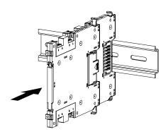
4) Push the sliders back into the body to fix the unit to the DIN rail.
