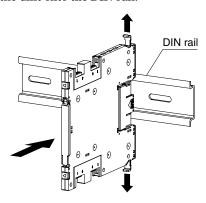
3) Push the sliders back into the body to fix the unit to the DIN rail.
