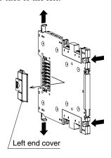
3) At tach the unit to be mounted onto the DIN rail while sliding $its\,male\,power\,connector\,along\,the\,female\,power\,connector$ of the already mounted unit so as to engage with each other. Confirm that the upper and lower tabs fit into the respective concave portions of the already mounted unit.
