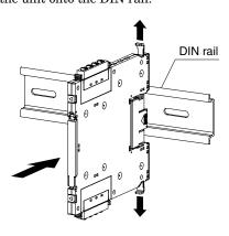
3) Push the sliders back into the body to fix the unit to the DIN rail.
