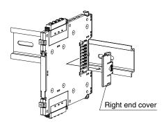
Remove the left end cover of the unit to be mounted next, pull out the upper and lower sliders, and slide the upper and lower tabs to the left.
