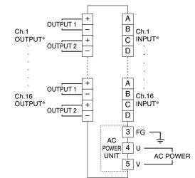
\*The input and output terminals are reversed for model M8YSx, M8YCx. Use either Output 1 or Output 2 terminal for the input.
