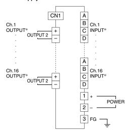
\* The input and output terminals are reversed for model M8YSx, M8YCx. Use either Output 1 (connector) or Output 2 terminal for the input.
