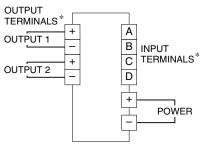
$^{st}$  The input and output terminals are reversed for model M8YSx, M8YCx. Use either Output 1 or Output 2 terminal for the input.
