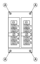
Mounting screws with washer for attaching power unit, M3 x 5 screws, 2 pls. per unit
