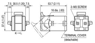
• 0 – 125A through 0 – 200A Use Sensor model No.: CLSB-20 Applicable cable diameter: Max. 24.0 Weight: 200 g (7.1 oz)
