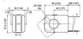
• 0 – 350A through 0 – 500A Use Sensor model No.: CLSA-50 Applicable cable diameter: Max. 36.0 Sensor leadwire: AWG 18, 200 mm Weight: 300 g (10.6 oz)
