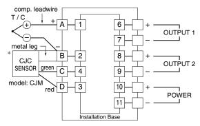
\*The CJC Sensor for the single mount base is not compatible with the one for the multiple mount base.
