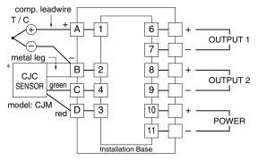
\*The CJC Sensor for the single mount base is not compatible with the one for the multiple mount base. Leadwires for the multiple mount type are replaced with metal legs with the single mount type.
